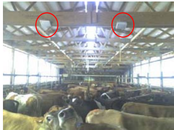
Figure 5. Sirit ID4100 circular polarized reader – dual antennas.
